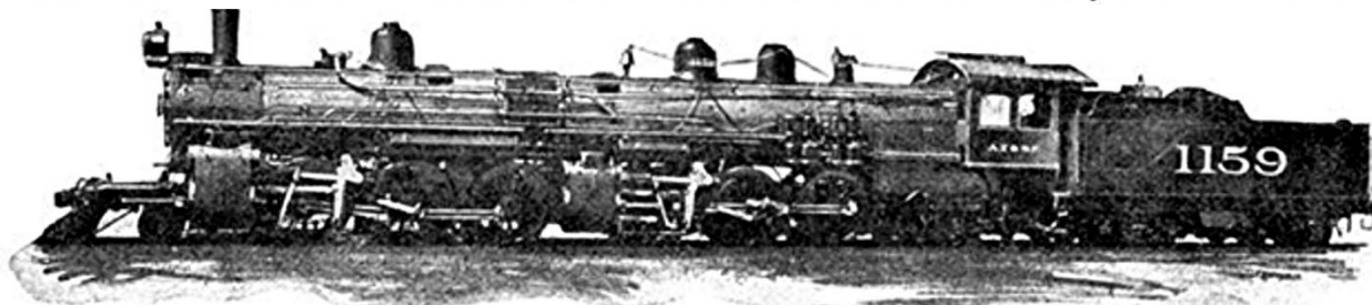
FIG 1 LOCOMOTIVE WITH FLEXIBLE BOILER BELLOWS TYPE OF CONNECTION
