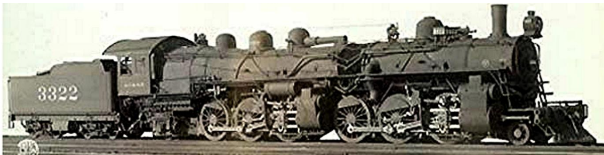
FIG 1 LOCOMOTIVE WITH FLEXIBLE BOILER BELLOWS TYPE OF CONNECTION
