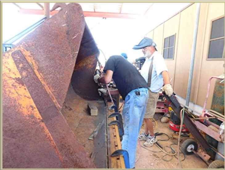
Scotty Brooks and Dave Griner putting a new cutting edge on the bucket of the newer tractor. Thank you both for the great welding job. The club is forever grateful for the very talented people that this club has.
