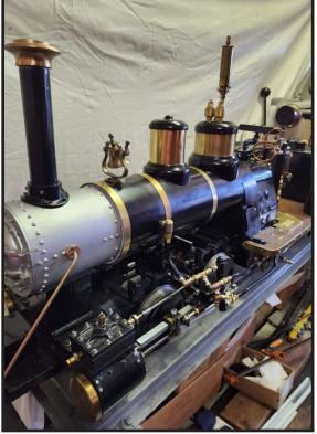
Engine detail without the cab shows piping for crosshead pump. Engine has been completely repainted.
