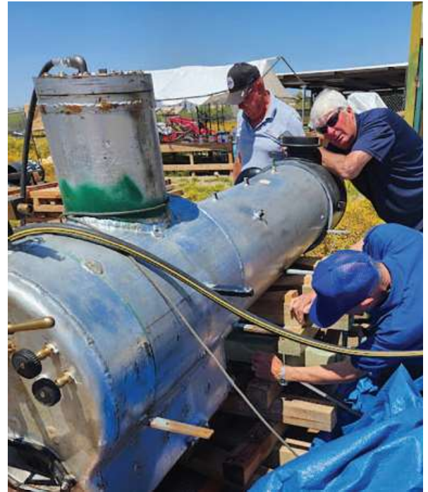
Terry L, Gary Gorman, president of Sahuaro Central, and Bob R. testing for leaks with water pressure.
