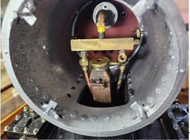
There is no pilot light on this loco, as there are only eight burners. Steam lines and header have been connected in the smoke-box. Steam line sealing packing is the round circle at the top of the flue sheet. Steam line with elbow is shown going into header.
