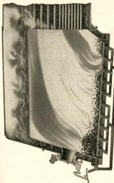
FIG. 4 Note hydrocarbon gases being distilled off from back of green coal under door. See how they escape unaccommodated for the most part when arch is not used. Also note how the fire and cold air rushing into lower flues, causing them to contract and leak.
