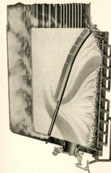
FIG. 5 Note how the arch deflects and mixes the shafts of cold air entering through the open fire-door and through holes in the fire. This mixing produces a more uniform temperature of the gases entering the flues and prevents the contraction of flues that causes them to leak.
