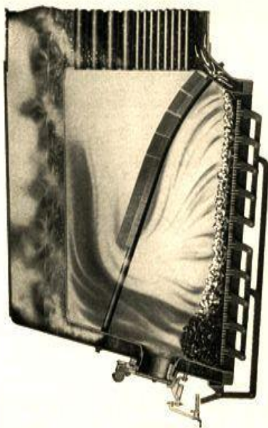
FIG. 2 Bank under fire-door reduces air supply through grates and reduces the temperature. Volume of hydrocarbon gases being driven off, thereby partly obscured.
