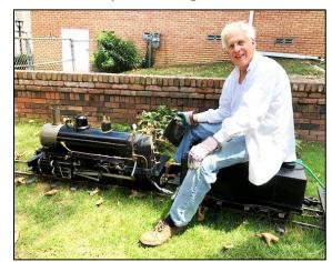
manner that can be easily maintained has taken the most thought and effort on this loco. It has powerful cylinders (also used on the LE 2-6-0 series) and will slip on start if one is not careful with the throttle.
