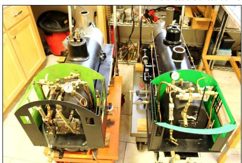
valve, steam brake valve, cylinder cock lever, reverser, throttle valve and whistle valve are in nearly the same relative locations. My blower setups use a triple valve-like arrangement to allow an air compressor to be connected until cutover to steam can be made. I use ball valves instead of globe valves for most controls as a convenience measure.
