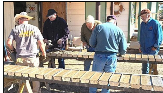
Pete Pennarts (and Perry McCully, cameraman) seen here training members on how to make cement ties.
