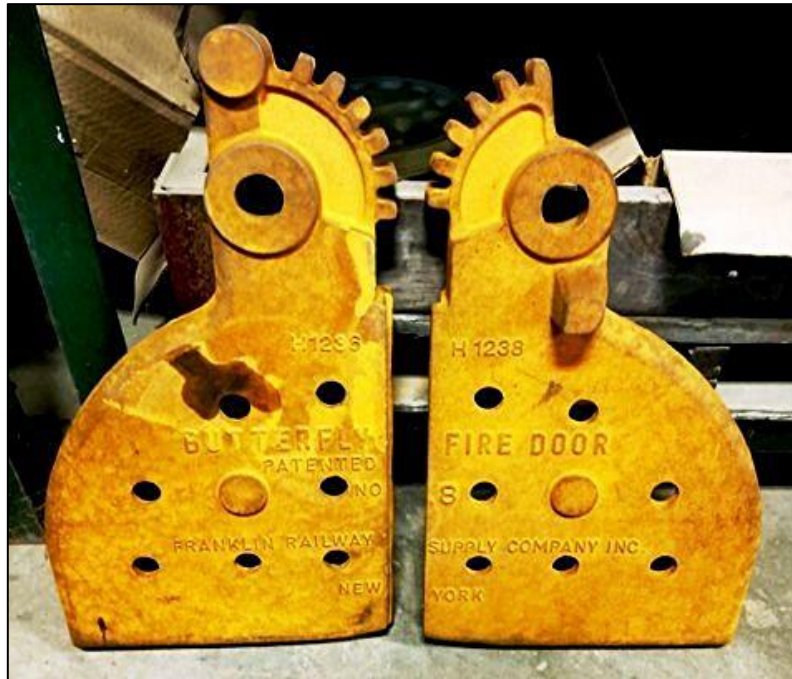
(left) Here are the left and right doors showing the gearing that makes them work simultaneously.
