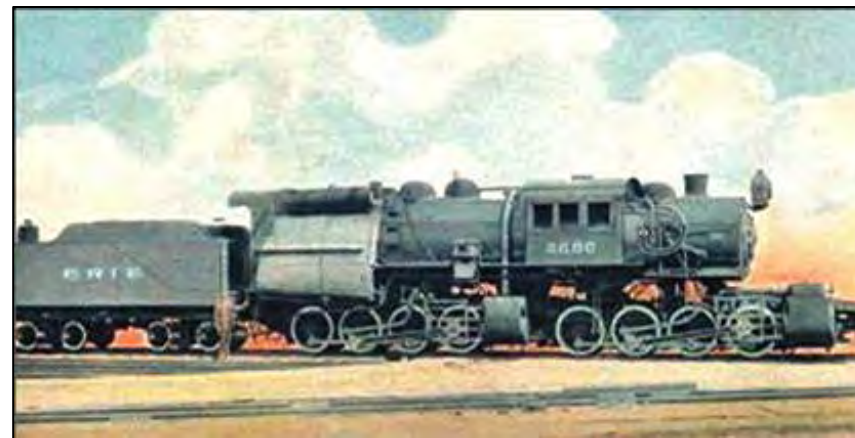
(right) No. 2600 was one of three articulated camelback locomotives built in 1907 by American Locomotive Co. for the Erie Railroad. Designed to handle grades in the Allegheny Mountains, they were replaced by larger engines in the 1930s. Painting by Unknown
