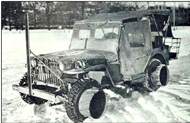
Winterization package (above) or with mud flotation adaptors (below).
