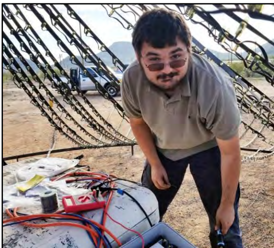
Timothy Freeman soldering new pixels on the megatree. There are 8,000 pixels (LEDs) on the tree.
