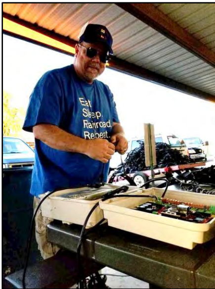
The new controller board was tested with the 50 foot cables to make sure the stars will light this year, and it works. This new board will also allow us to place the mini trees closer to the tracks. And it still has room for future expansion.
