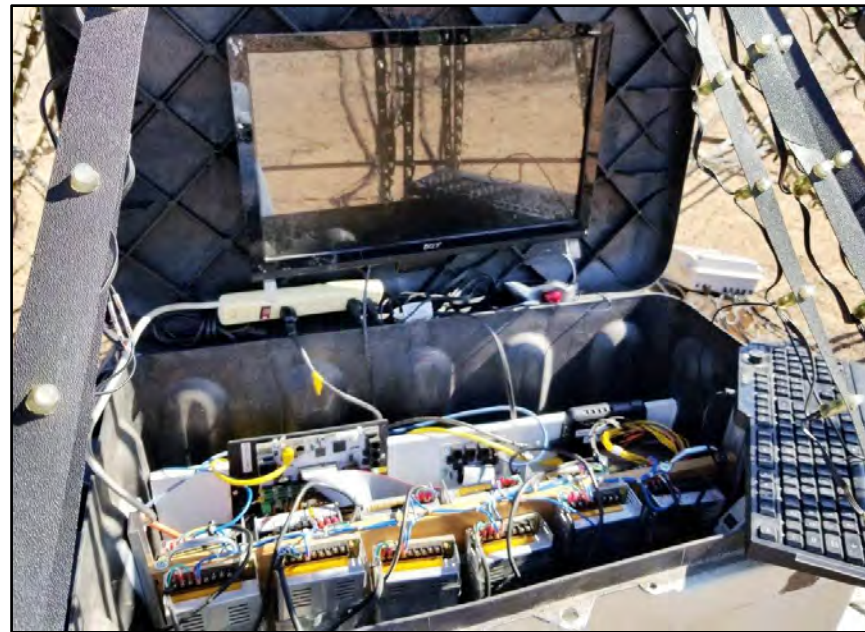
Here is the gem that runs the Megatree, a Falcon F16 pixel controller running from a micro PC.
