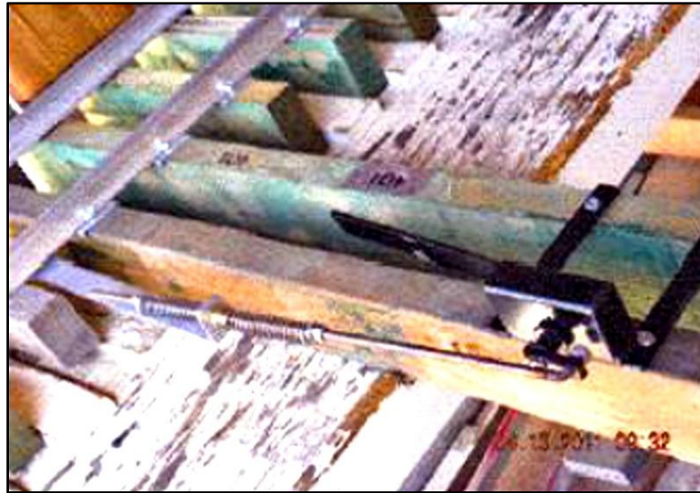
The throw mechanism for switch number 401.
