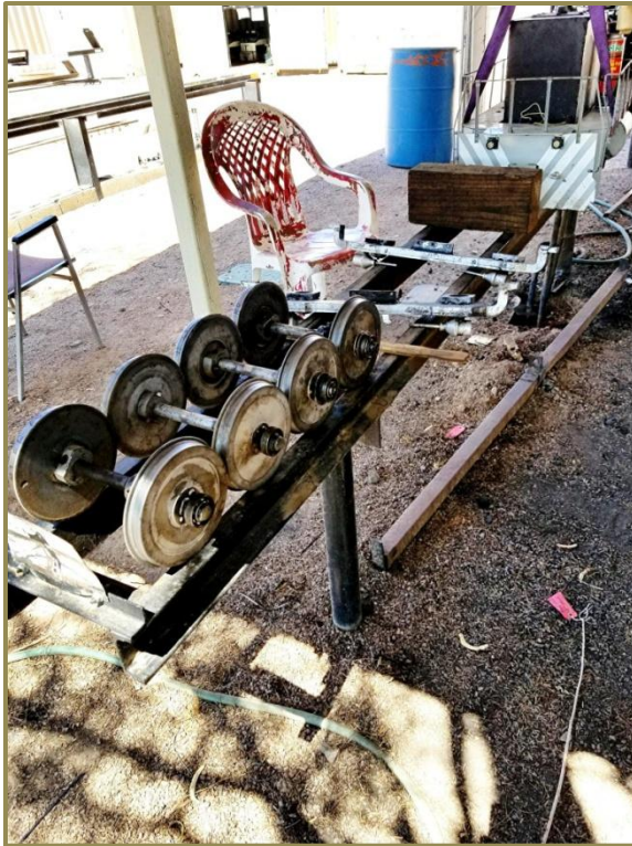
MLS locomotive UP 2001 getting ready for new wheels.
