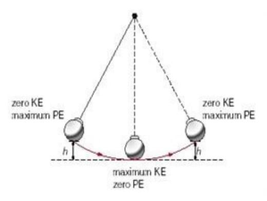
The drawing shown above denotes the swing of a pendulum. This duplicates the action of all of the components in this gear. The most significant concept is to understand how, as the rod swings from its intersection with the tangent, there is a displacement of the ball end relative to the tangent line, shown here as the distance "h".
