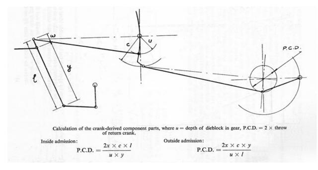
Here is another example, as shown in developing the movements of the combination lever and expansion link.
