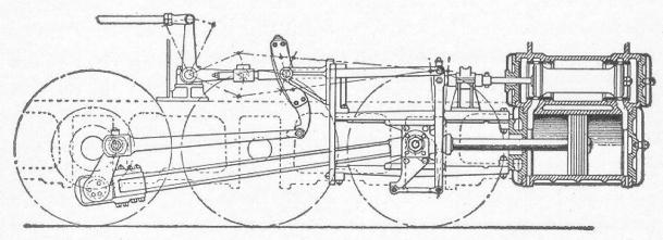
Fig. 68-b. Walschaert Gearing Mounted on a Consolidation Locomotive.
