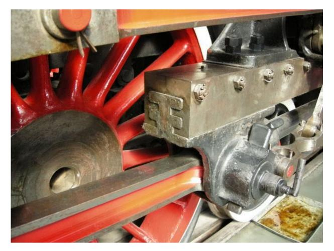
This is a more modern method using what is referred to as a multiple bearing crosshead. Looking closely we can see the end of the guide and it six major points of bearing. Have been involved in re-babbitting one of these for a large 4-8-4 using straight tin, preheating the casting to 500 dg F, tinning the surfaces, then pouring the tin, it was an exciting event!!
