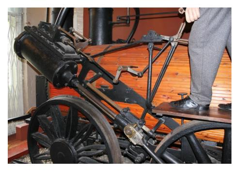
These guiding bars can be found in a variety of configurations, for instance one above, one below the piston rod as illustrated below. At this point it should be noted that the effort exerted by the piston rod through the main rod puts the load on the upper guide bar when the engine is running in the forward direction, the lower bar when in reverse.
