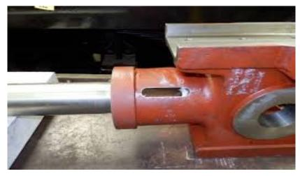
This is the piston rod key slot ready for the key to be driven, pulling the rod into the crosshead hence the necessity for really accurate machining.
