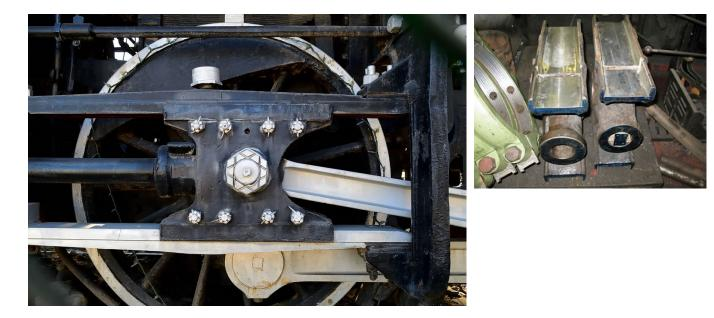
The picture above shows the guiding surfaces (slippers), along with the tapered piston rod collars. Typically the slippers are a Babbitted surface. You can see an arrangement to lay out the center of the bore on the collar in preparation for machining the fit of the piston rod.
