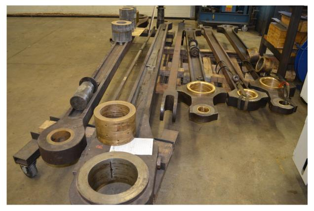
The strap and wedge was always a problem waiting to happen where the strap had a tendency to break, causing the rod to fail about and to allow the piston to slam into the cylinder head. The following design removed this problem and provided better wear characteristics, where the bearing rotated in a steel sleeve inserted into the rod end. The strap has been eliminated and the rotational speed of the bearing relative to the crank pin is reduced, thus reducing wear. This
