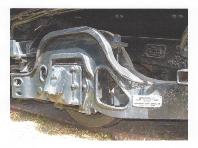
This was a free swinging design having a tongue attached at the rear of the frame and supported at the rear of the truck by heart rockers. You can see the truck has its own springing.
