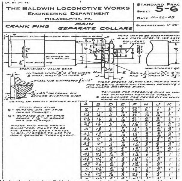
This drawing shows how Baldwin went about the design of crankpins and how much pressure was required to set them properly into the driving wheel center. It might also be interesting to note the pin has provision for being riveted over at the rear. Close attention was given to providing generous radii to prevent stress raisers from developing due to corners where diameters changed.
