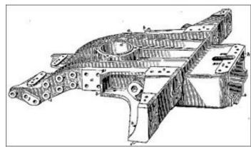
Typically the front of the frame is held by the pilot beam and the cylinder structure.
